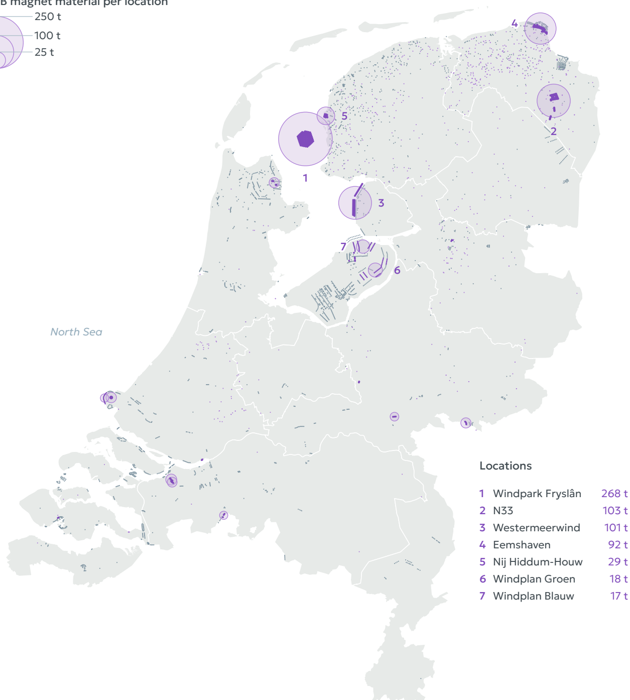
Figure 2 | Dutch onshore wind turbines with and without NdFeB magnets in the main generator, and the magnet material per location. The area of a bubble is proportional to the magnet material of a location in the central estimate, for locations with at least 5 tonnes. Map based on CBS (n.d.-a, n.d.-b).
